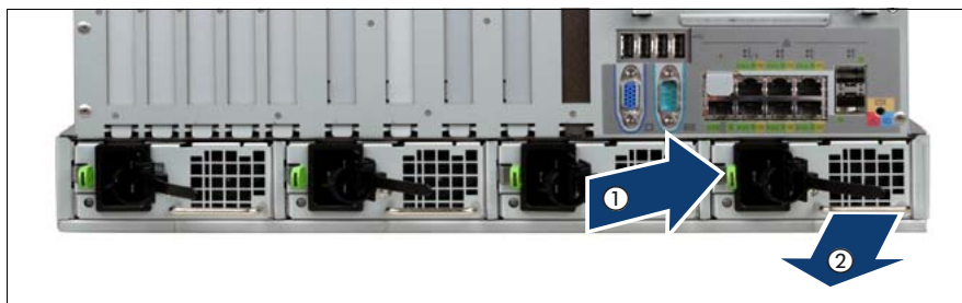
Figure 15: Unlocking and removing the power supply unit
